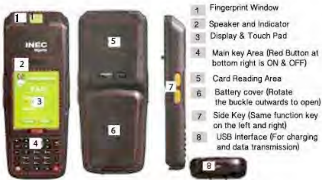
Fig. 2.2 Features of the Smart Card Reader
